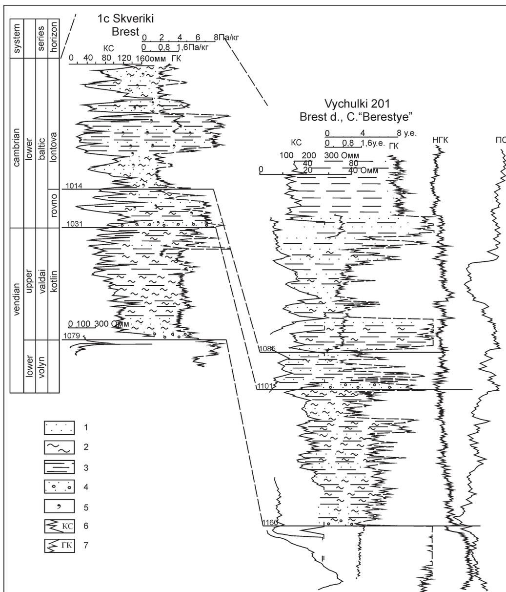
**Figure 43.** Vendian–Cambrian boundary in the boreholes Skweriki-1c [4] and 201 Vychulki-201 drilled near Brest. Legend: 1 – sandstones, 2 – siltstones, 3 – mudstones, clays; 4 – gravelites, 5 – glauconite, 6 – apparent resistivity log (KC), 7 – Gamma Ray log (ГК).
